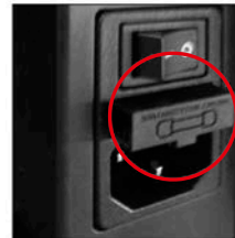
Picture 5: The fuse cartridge slides out towards you.
