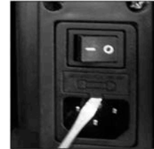
Picture 4: Unhinge the fuse cartridge with a flathead screwdriver.
